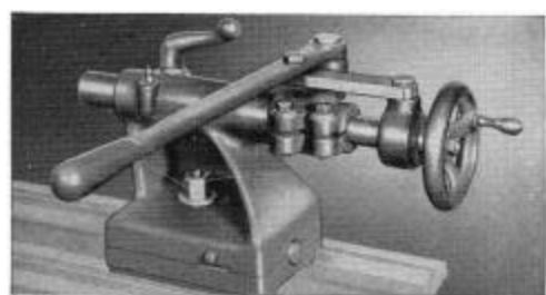
AC-241 LEVER TAILSTOCK ASSEMBLY Can be furnished with the Quick Change Gear Lathe in place of tailstock shown in above illustration of the lathe if specified in your order. Lever stroke, 2 3/4". Hand wheel spindle travel, 2 3/8". Fitted for No. 2 Morse Taper Shank.
